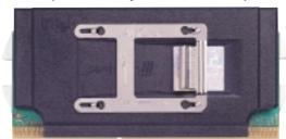
Example of an incorrectly installed retention clip
